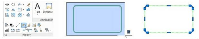
• Type O and press Enter. Type 25 and press Enter to define the offset distance. Select the polyline and click in the area enclosed by it. Press Esc.
