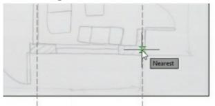
• Select the horizontal grid line and drag the endpoints to stretch it outside the image.
