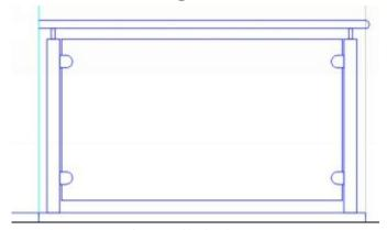
• On the Status bar, click the **Polar Tracking** icon. Click the down arrow next to the **Polar Tracking** icon and select 30. Activate the **Line** command and create an inclined line, as shown. Offset the inclined on both sides. The offset distance is 100 mm.
