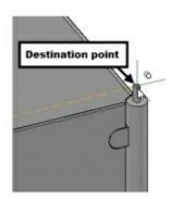
Type PL and press Enter. Select the center points of the top face of the posts, as shown.
