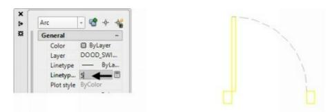
• On the ribbon, click **Home** tab > **Layers** panel > **Layer** drop-down > **A-WALL**. Create two vertical lines of 320 length, as shown.
