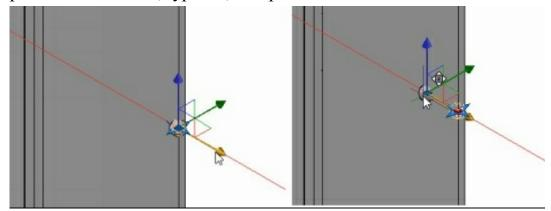
Select the Y-axis (green arrow) of the Move Gizmo and move the sphere forward. Type 25 and press Enter. Press Esc to deselect the sphere.
