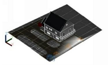
Select the rectangular array, click on the Z-axis of the move gizmo, and move the pointer upward. Type 6100 and press Enter.
