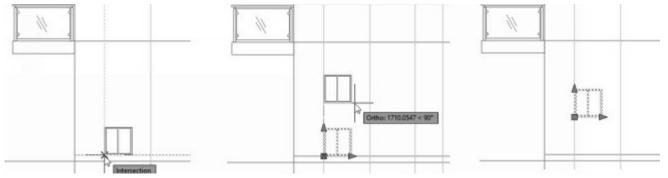
• Use the arrow grips of the window block to set its width and height.
