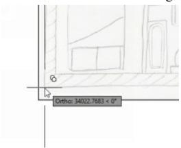
• On the **Home** tab of the ribbon, expand the **Draw** panel and click the **Construction Line** icon.
