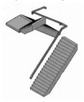
Create an 80x80x1050 box on the bottom stair, as shown. Move the box 10 mm towards right and 69 mm backwards.
